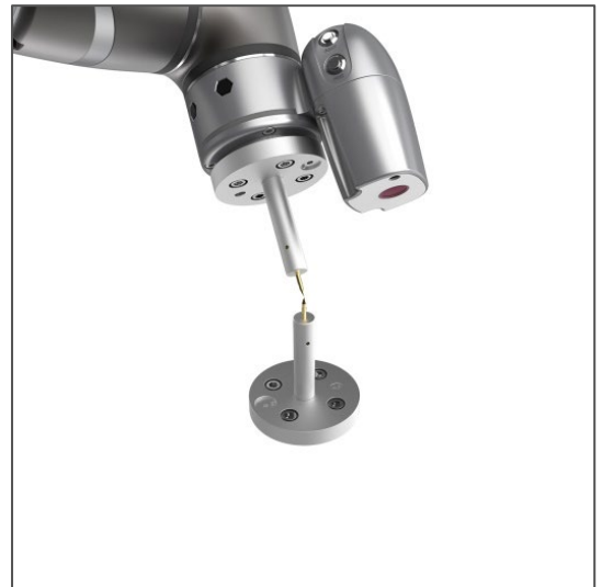
Figure 108: The Robot Posture Needs to Change during Teaching (1/2)
