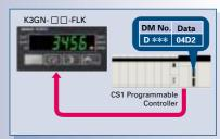
The model that is equipped with communications capability enables you to display data from PLCs or PCs directly.
