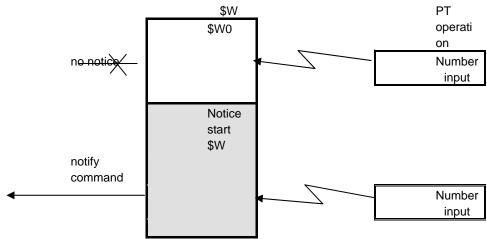
Only changes from specified \$W number and up are communicated to host using the change notice Command.
