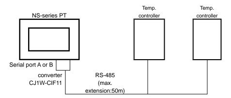
By using another communications port, you can simultaneously connect temperature controllers and a host. With one more serial port, NS can connect PLC, barcode reader, Memory Link and can communicate with CX-Designer.
