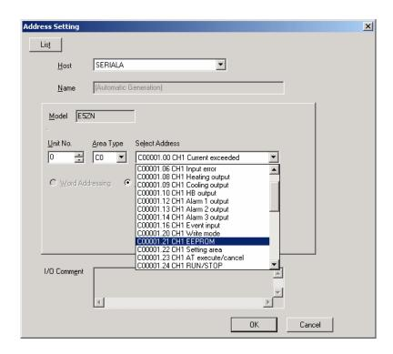
You can also manually enter a communications address, which is not listed without opening Address Setting dialog. In this case, enter the desired address directly to the field shown in the property dialog.
