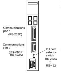
Two types of connectors are provided to CV500-LK201 host link unit. Both of these connector types can connect to the NT620S/620C with an RS-232C connector cable. Select the connector cable which matches the connector type.
