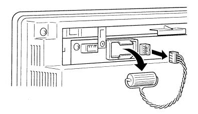
4. Install a new battery. Insert the battery connector, keeping it straight.
