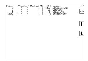
For both order of occurrence and order of frequency, the number of entries that can be displayed on one screen is 23 in the case of the NT620S and 27 in the case of the NT620C.
