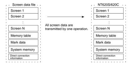
When screen data is transmitted from the support tool to the NT620S/620C, all existing screen data in the NT620S/NT620C is deleted.
