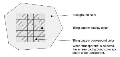
Part of the graphic frame may be invisible because of the combination of the display (in filling), background and outline colors. This phenomenon is peculiar to a color LCD, not a failure with the system.
