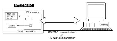
Seen from the perspective of the NT620S/NT620C, when using the memory link method it makes no difference whether the "object" communicated with in direct connection is external or internal, and therefore screen data for direct communication can be used without alteration by merely changing the object of communication.
