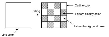
When a lamp, a touch switch and a graphic are to be displayed in specific colors, part of the frames of the display elements may be invisible because of the combination of the background, outline and filling colors. This is a phenomenon peculiar to a color LCD, not a failure with the system.
