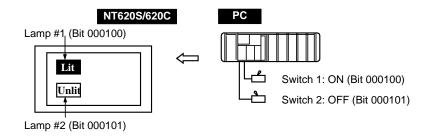
PC's bit status is displayed by the "Lamp" on the NT620S/620C.
