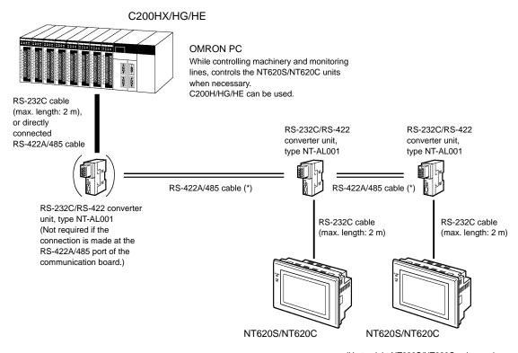
(Up to eight NT620S/NT620C units can be connected.)
