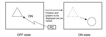
For the Image Library LAMP, presence of external frame, Lit/Flashing, color display, guide display, and so forth cannot be specified, unlike normal LAMP.
