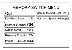
Each time the "Key Press Sound" touch switch is pressed, the setting option "ON" alternates with "OFF".
