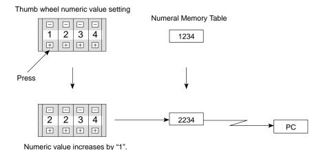
A numeric value cannot be entered into the thumb wheel type from the ten-key.
