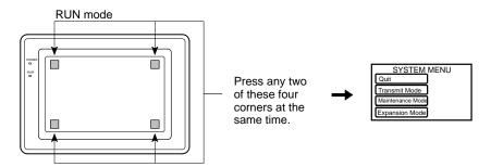
Note that the touch switches used to call the System Menu are not displayed on the screen. If a touch switch displayed in a corner is pressed first, the touch switch will function and the System Menu will not be displayed. To successfully call the System Menu, first press a corner where no touch key is displayed, and then, press any other corner regardless of the presence of a touch key.
