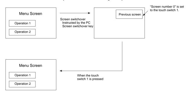
Only a touch switch can have the screen switchover return key function. If display of screen number "0" is specified from the PC, the screen will go blank.
