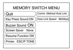
Each time the "Host Link Speed" touch switch is pressed, the setting option "9600 bps" alternates with "19200 bps".
