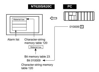
When the PC bit comes ON (1), the contents of the character-string memory table registered for the bit memory table are displayed in the alarm list. When the bit returns to the OFF (0) status, the character-string memory table display is automatically cleared.
