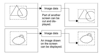
Image data of up to 224 images can be registered in a screen data file as code of FE20 to FEFF.
