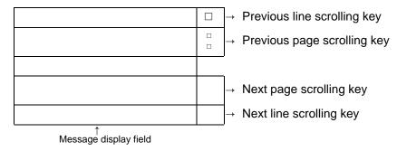
When the number of lines for message display is set to one to three, only line scrolling keys are automatically created.
