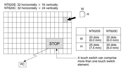
When the touch switch is pressed, its information is sent to the PC.
