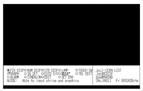
Create screen data in the Edit screen of the support tool. Data of one screen can be created by registering (laying out) the following display elements and attributes on the screen.
