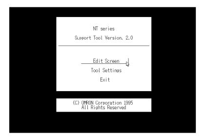
Select "Tool Settings" in the Main Menu to display the "Tool Settings" screen. Settings of NT model, memory size, direct connection, etc. are made in this screen. Refer to "Setting the support tool for use with the NT620S/620C" on the previous page.
