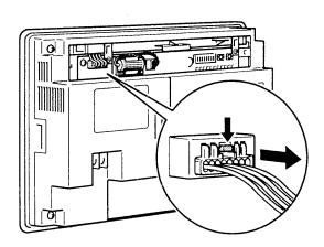
3. Remove the screws that secure the backlight with a Philips head screwdriver, grip the handle, and pull the backlight out (note that the screws are designed not to come out of the backlight). As shown in the figure below, the backlight can be removed easily if it is pulled straight out to begin with and then at a downward angle.
