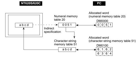
This specification method is a little complex, but it allows the display to be changed more easily according to the circumstances. In the example above, if 1
