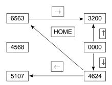
When the HOME key is pressed, the cursor can be moved at a stretch to an area at the upper left corner where a sum of XY coordinates is at a minimum (the numeral setting input column at the upper left in the example above).
