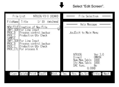
Select a file used for storing the screen data for the NT620S/620C in the "File List" screen.
