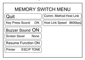
Each time the "Printer" touch switch is pressed, the next item in the applicable cycle of options below is selected:
