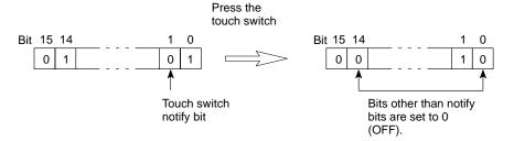
In the case of (2) in the table, since notification is executed on the basis of the contents of the word before display, the other bits in the word are not overwritten. However, if the contents of the word are changed at the PC during display, they will be rewritten based on the contents before display.
