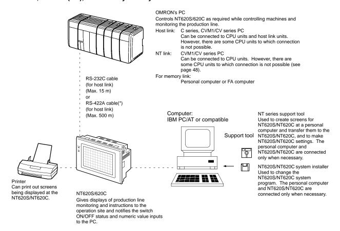
\* When the NT620S/NT620C is used with RS-422A, an RS-232C/RS-422 converter unit (NT-AL001) is required.
