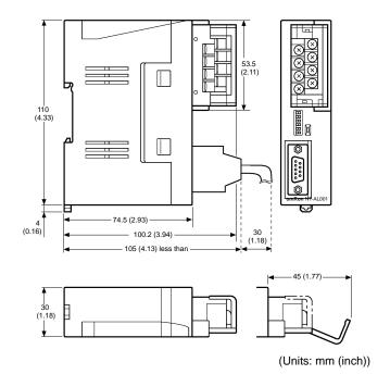
With RS-422A terminal block cover closed: 30 (W)  $\times$  114 (H)  $\times$  100.2 (D) mm With RS-422A terminal block cover open: 30 (W)  $\times$  114 (H)  $\times$  119.5 (D) mm
