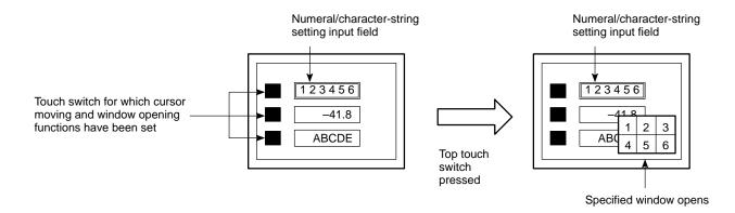
If the cursor moving keys are created automatically during creation of a numeral/character-string input field with the support tool, the window opening function is not set. In this case, the window to be opened can be specified by modifying the touch switch.
