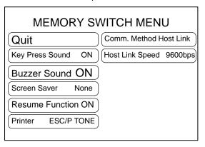
Each time the "Screen Saver" touch switch is pressed, the setting option will switch among "10 minutes", "1 hour", and "None".
