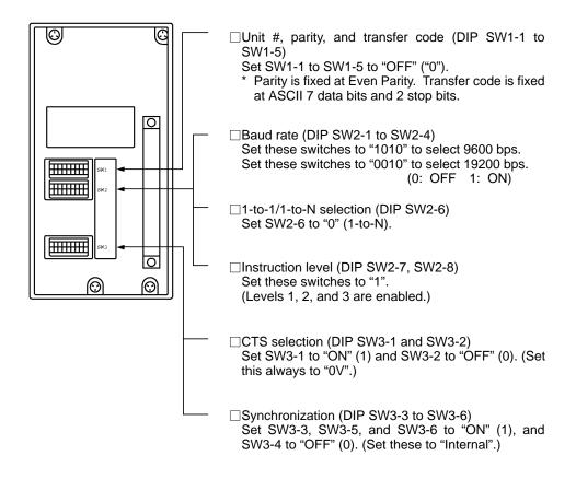
□CVM1/CV series backplate mounted type: CV500-LK201
