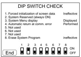
After checking the DIP switch statuses, press the "End" touch switch.
