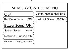
Each time the "Resume Function" touch switch is pressed, the setting option "ON" alternates with "OFF".
