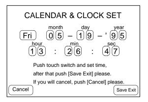
The "CALENDAR & CLOCK SET" screen will be displayed (it will display the time at the instant the "Set" touch switch was pressed).
