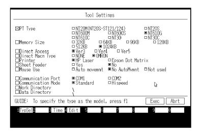
To create the NT620S/620C screen data, make settings in the "Tool Settings" screen as follows.
