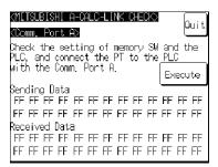
To execute checking, press "Execute". The data is transmitted to the host for checking the communication and displayed on "Sending Data" in hexadecimal.
