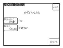
Press the "Connect Model" and "Comm. Speed" to select the type of the host to be connected and the communication speed. The display on the right of each touch switch will be changed by pressing the switch.
