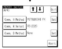
Press the touch switch of the port ("Comm. A Method" or "Comm. B Method"), to which the computer link system that uses Mitsubishi A series PCs is to be set, to display "MITSUBISHI FX".
