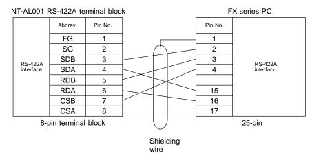
Make the connections between SDA and SDB, RDA and RDB, and CSA and CSB, with twisted pair wires.
