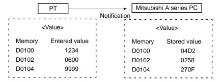
**(Example)** When the value representation at the PT side is specified to "binary", the value is entered at the PT side:
