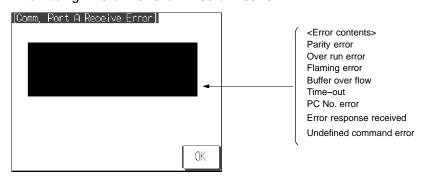
The errors that occur specifically with computer link systems that use Mitsubishi A series PCs are described below. For details on errors other than those indicated below, refer to the Operation manual for the PT.
