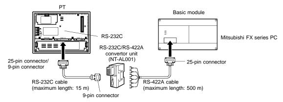
**Notice:** • After connecting a communication cable, always secure it with the screws.
