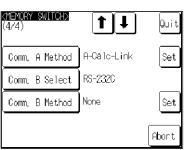
Press the touch switch of the port ("Comm. A Method" or "Comm. B Method"), to which the computer link system that uses Mitsubishi A series PCs is to be set, to display "A-Calc-Link".
