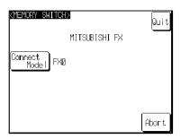
Press the "Connect Model" to select the type of the host to be connected.
