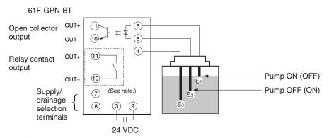
Note: The part within the dotted-line box is for the 61F-GPN-BC (relay-output type) only.
