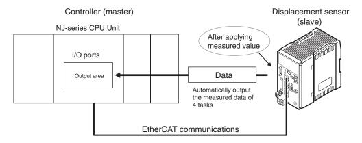
With EtherCAT communications, communications is performed via the I/O ports of the following four area on the Controller. Sysmac error status area I/O ports are used only when an NJ series CPU unit is connected as the master.
