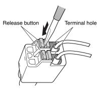
3 Reinstall the 24 V input terminal block to the Sensor Controller.
