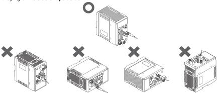
For adequate intake and/or exhaust, keep the Sensor Controller clear by 30 mm or more on its top, and by 10 mm or more from either side.
