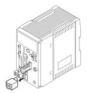
2 Push in and hold the release button next to the terminal hole using a screwdriver while pushing the wire fully into the terminal hole and remove the screwdriver.
