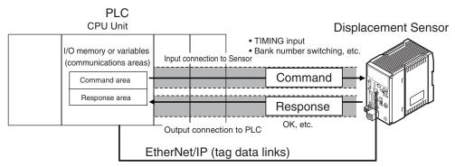
To send a control command, you write a control command to the command area (i.e., a variable or I/O memory address in the PLC) that is specified for the output tag, and then turn ON the Command Execution (EXE) Bit. As a result, the control command is sent through the input connection from the PLC to the Displacement Sensor.
