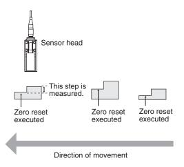
The zero reset function also allows setting the reference value to the hold value for a hold measurement or any value other than zero.
