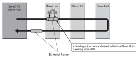
It is the "EtherCAT datagram" stored directly in an Ethernet frame that exchanges data regularly between the EtherCAT Master Unit and Slave Units.
