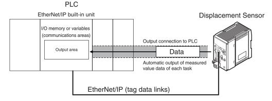
To output data, specify the I/O memory area or a variable (output area) on the PLC for storing that data in advance to the input tag.
