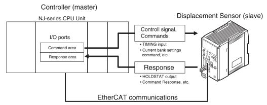
The Controller sends the instruction to the displacement sensor over EtherCAT by switching the control signal bit assigned with control to be executed to ON.
