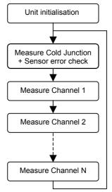
The cold junction compensation measurement and one sensor error check are executed each cycle.
