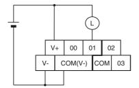
Although V- and COM(V-) are connected internally, also wire them externally.
