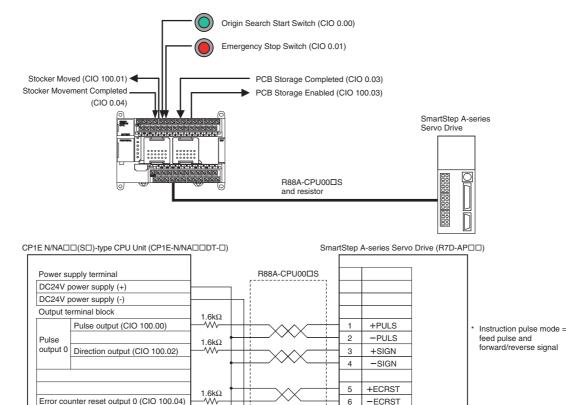
Only N□□S(1)-type CPU Units can wire V+ and V-. Do not wire them in N□□-type CPU Units.
