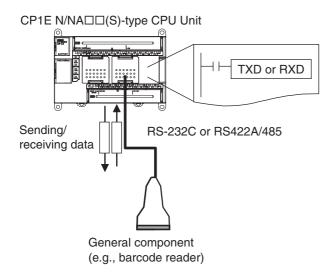
No-protocol communications are used to send data in one direction to or from general external devices that have an RS-232C or RS-422A/485 port using TXD or RXD.
