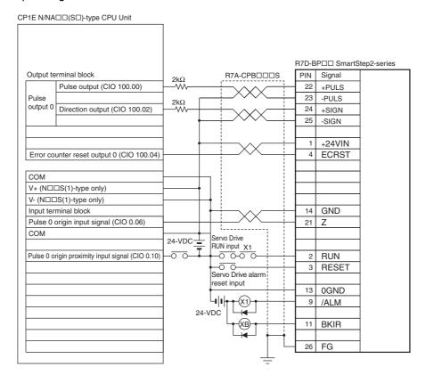
Only N□□S(1)-type CPU Units can wire V+ and V-. Do not wire them in N□□-type CPU Units.
