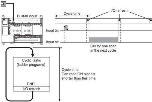
The pulse widths of quick-response input signals must meet the following conditions.
