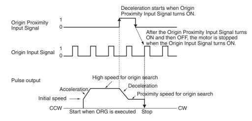
Origin Detection Method 1: Origin Proximity Input Signal Reversal Not Required
