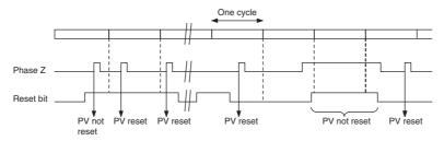
Note The phase-Z signal cannot be used if an incremental counter is specified. Only a software reset can be used.
