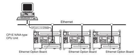
Executing, from the host computer, FINS commands with UDP/IP or TCP/IP headers enables various control operations, such as the reading and writing of I/O memory between PLCs, mode changes, and file memory operations.
