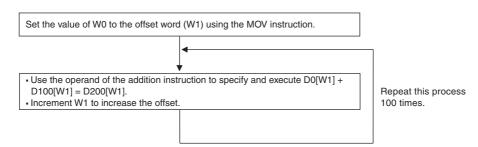
Each process is performed with an input comparison instruction (<) as the execution condition so that W1 does not exceed &100 to make sure that the upper limit of the indirect addressing range is not exceeded.
