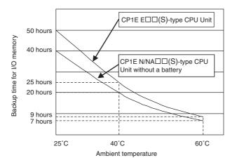
The following areas are unstable when power is interrupted for longer than the I/O memory backup times given above.
