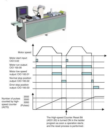
While the pulse count is between 3,500 and 3,550, normal stop position output (CIO 100.02) will be ON. If the pulse count exceeds 3550, the error stop position output (CIO 100.03) will turn ON.
