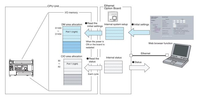
Note The initial settings of the Ethernet Option Board cannot be set in the allocated words in the DM area or in the CX-Programmer's system settings.
