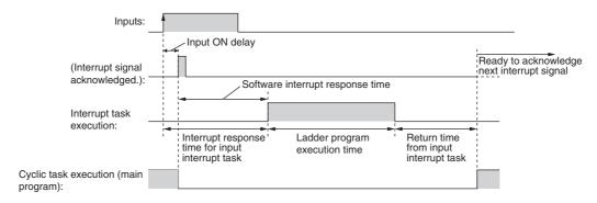
The time from when execution of the input interrupt task is completed until execution of the cyclic task is resumed is 24  $\mu s.$
