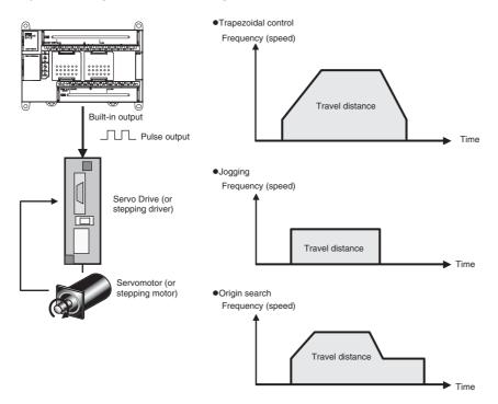
Positioning is performed with a servomotor or stepping motor in the following configuration.
