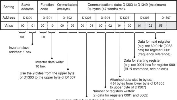
Register number for starting data write: 0001 (Specifies to start writing data to Inverter starting at register 0001.)
