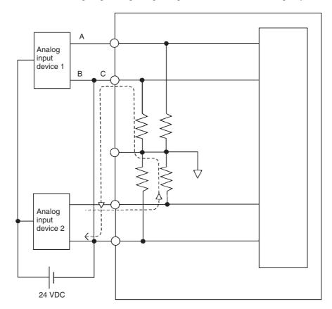
5 Refer to the following diagram regarding wiring disconnections when voltage input is being used.
