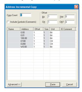
2 In the Offset Area set the Bit Field to 16 and the CH Field to 10 for this example.
