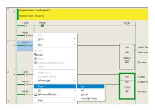
The input bit will be force-set. A symbol indicating the force-set status will be displayed at the input condition.
