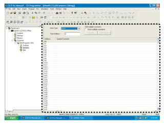
2 Input I/O comments or double-click the address for which the I/O comments are to be changed. Inputting the I/O comment will be enabled, so input the I/O comment.
