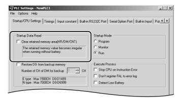
Note If the Restore D0- from backup memory Check Box is selected, only the specified words in the DM Area will be restored from the built-in EEPROM backup memory when the power supply is turned ON.
