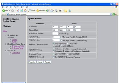
6 Select 1. IP address and Protocols - System to display System menu.
