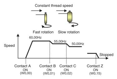
The target speed is changed according to inputs from multiple contacts. Acceleration and deceleration are controlled using the acceleration and deceleration of an inverter.
