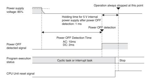
Power OFF Detection Time: The time from when the power supply voltage drops to 85% or less the rated voltage until the
