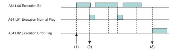
(1)Turn ON A641.00 (Execution Bit) to send command data stored starting at D1300. For details, refer to DM Area Data on page 14-19.
