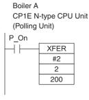
Transfer CIO 2 and CIO 3 to CIO 200 and CIO 201 using a BLOCK TRANSFER instruction. Boiler B CP1E N-type CPU Unit (Polled Unit No. 0) P On XFER #2
