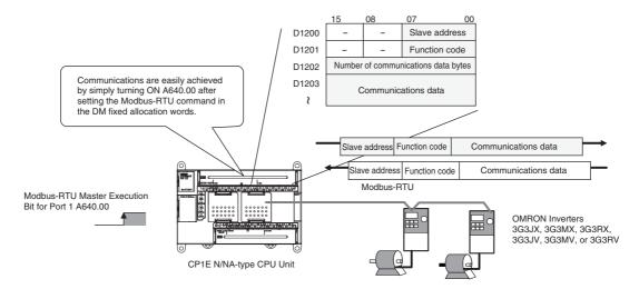
Modbus-RTU commands can be sent simply by turning ON a software switch after setting the Modbus slave address, function, and data in the DM fixed allocation words for the Modbus-RTU Easy Master. The response when received is automatically stored in the DM fixed allocation words for the Modbus-RTU Easy Master.
