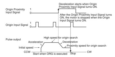
• Origin Detection Method 2: Origin Proximity Input Signal Not Used
