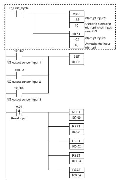
The MSKS instruction is used to specify an interrupt when the input turns ON and then it is used to unmask the input interrupt.
