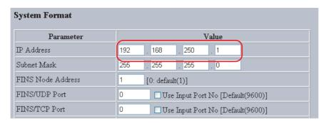
**8** After entering the correct values, click the Transfer Button to transfer the settings to the Ethernet Option Board.
