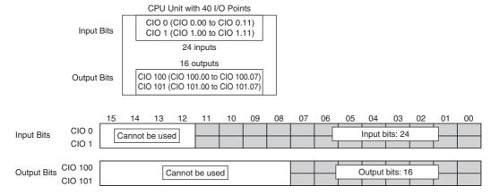
For a CPU Unit with 40 I/O points, a total of 24 input bits are allocated to the input terminal block. The bits that are allocated are input bits CIO 0.00 to CIO 0.11 (i.e., bits 00 to 11 in CIO 0) and input bits CIO 1.00 to CIO 1.11 (i.e., bits 00 to 11 in CIO 1).
