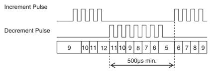
• Cycle time exceeded error occurs when using target matching When using target matching, if the encoder input values change fast due to vibration, the direction changing may be at a high frequency, cycle time exceeded error may occur as a result. At this time, take measures to stabilize the encoder inputs or use range comparison.
