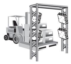
• If a point where the RF Tags are unreadable (null point) is generated due to the cancellation (multi-path) of the radio waves due to reflected wave in the ambient environment, RF Tag communications will be possible at high reading accuracy if multiple Reader/Writers are arranged, supplementing the null point.
