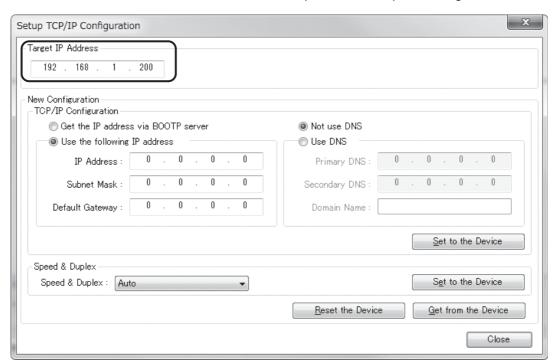
Enter the default IP address of the Reader/Writer (192.168.1.200) in the Target IP Address Box.
