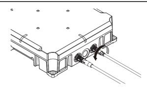
Hold onto the connector on the Power Cable and pull it straight out to remove it.
