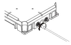
Hold onto the connector on the Ethernet Cable and pull it straight out to remove it.
