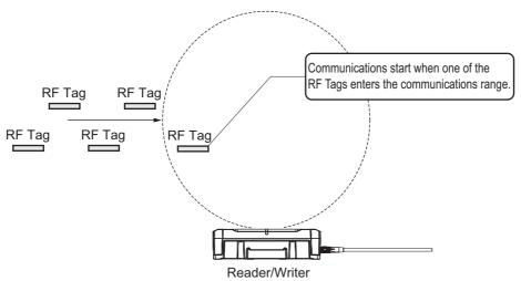
The Reader/Writer waits for multiple RF Tags to enter the communications range, and starts communications even if one RF Tag is detected. Each time the communications process is completed, the Reader/Writer returns a response. The communications operation continues until the command execution request from the host device is cleared.
