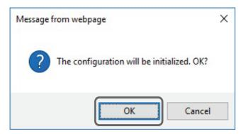
The following information is displayed after setting is completed. The network settings (NetworkSetting) are applied when the Reader/Writer is restarted. The RF Tag communications settings (RFCommunicationSetting) are applied immediately.
