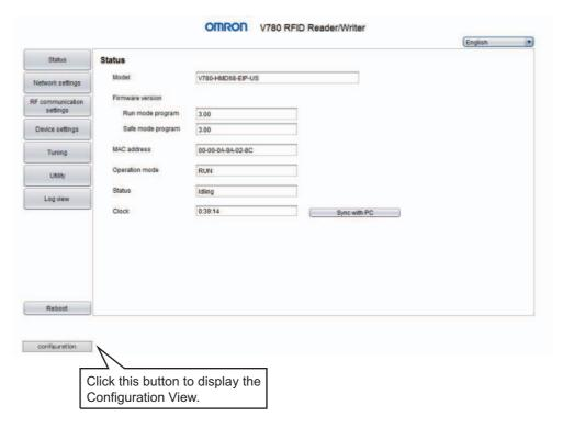
Click the Configuration Button to display the Configuration View.
