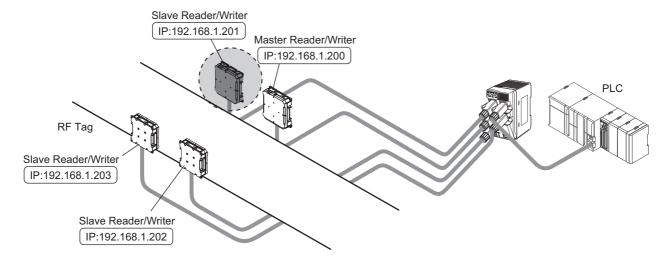
After the communications process of the Slave Reader/Writer comes a full circle, the operation is repeated from step 2. If the timeout time elapses during the communications process, a response (RF Tag Missing error or RF Tag communications error) is returned to the host device, and the processing ends.
