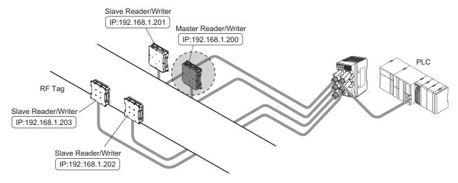
Slave No. 1 will communicate with the RF Tags with the "Once" communications option. Here, if the communications have ended normally, or if the communications have ended with an error, a response is returned to the host device, and the processing ends. If an RF Tag Missing error or an RF Tag communications error is detected, the processing will continue in the order of Slave No. 2, Slave No. 3.
