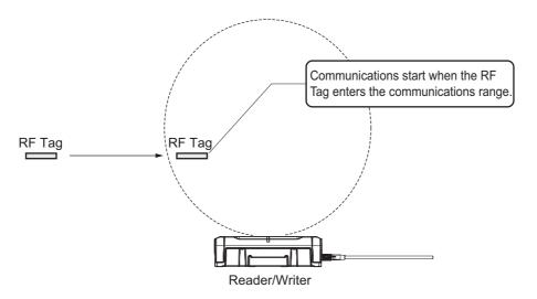
The Reader/Writer waits for an RF Tag to enter the communications range and returns the communications results after it detects an RF Tag. If there is already an RF Tag in the communications range when the command is executed, the Reader/Writer communicates with the RF Tag.
