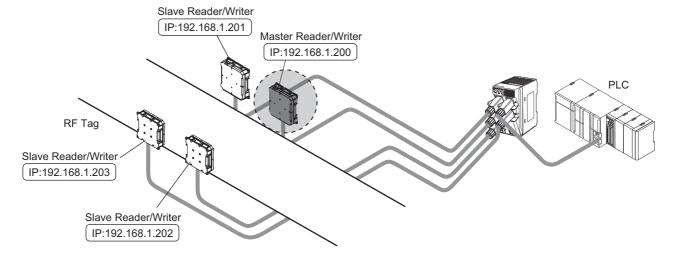
Slave No. 1 will communicate with the RF Tags through the "Once" communications option. Here, if the communications have ended normally, the communications results are returned to the host device. If the communications results indicate an RF Tag missing error or a communications error, an error response is not returned to the host device, but if any other error is detected, the error results are returned to the host device. The processing will continue in the order of Slave No. 2, Slave No. 3.
