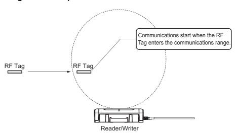
The Reader/Writer waits for an RF Tag to enter the communications range and returns the communications results after it detects an RF Tag.
