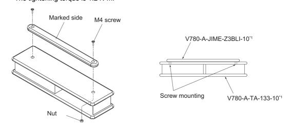
**2** Mount the Attachment to which the RF Tag is mounted to the metallic material. Mount it with two M4 bolts.
