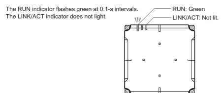
The RUN indicator lights when the Reader/Writer starts in Run Mode, and a connection of the tag data link from the originator is established.
