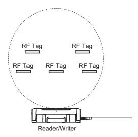
· One or More RF Tags in the Communications Range If the Reader/Writer detects more than one RF Tag within the timeout time, it waits for the timeout and then returns the communications results. Communications results are not returned for RF Tags that could not be communicated with within the timeout time.
