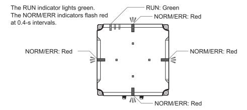
Illegal Network Setting or Incorrect Operating Mode Detection during Operation
