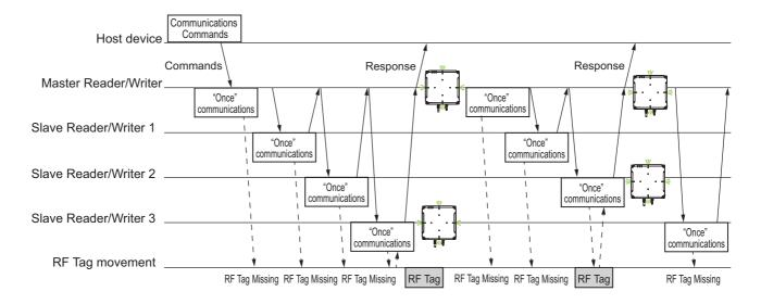
· If the RF Tag completes normally in any of the Reader/Writers in multiaccess
