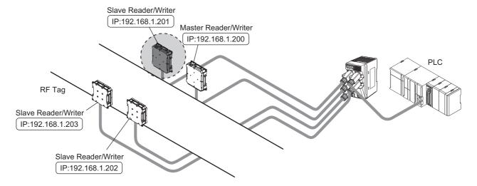
After the communications process of the Slave Reader/Writer comes full circle, the operation will be repeated from step 2.
