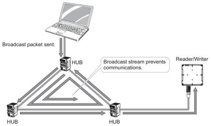
Also, if a large volume of broadcast packets or multicast packets are placed on the network, the Reader/Writer's response speed will drop and the Reader/Writer may even stop operating. Do not place a large volume of packets on the network in this way. Also, separate segments for the Reader/Writer from broadcast or multicast packets.
