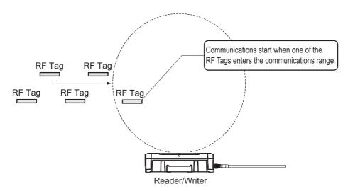
After the command from the host device is executed, the Reader/Writer automatically detects any RF Tags that enter the communications range and starts communications when even one RF Tag is detected. If the Reader/Writer then detects more RF Tags within the timeout time, it waits for the timeout and then returns the communications results. Communications results are not returned for RF Tags that could not be communicated with within the timeout time.
