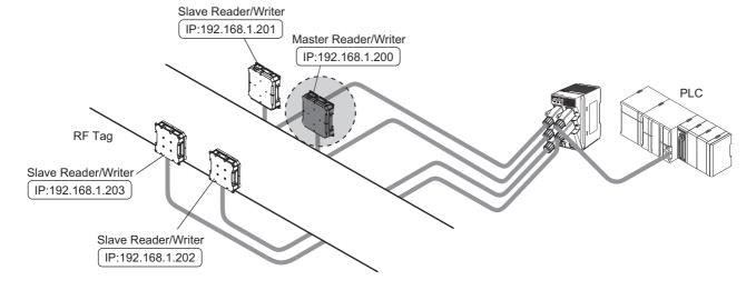
Slave No. 1 will communicate with the RF Tags with the "Once" communications option. Here, if the communications have ended normally, or if the communications have ended with an error, a response is returned to the host device, and the processing ends. If an RF Tag Missing error or a communications error is detected, the processing will continue in the order of Slave No. 2, Slave No. 3.
