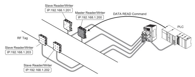
The master Reader/Writer will communicate with the RF Tags with the "Once" communications option. Here, if the communications have ended normally, or if the communications have ended with an error, a response is returned to the host device, and the processing ends. If an RF Tag Missing error or a communications error is detected, it will progress to step 3.
