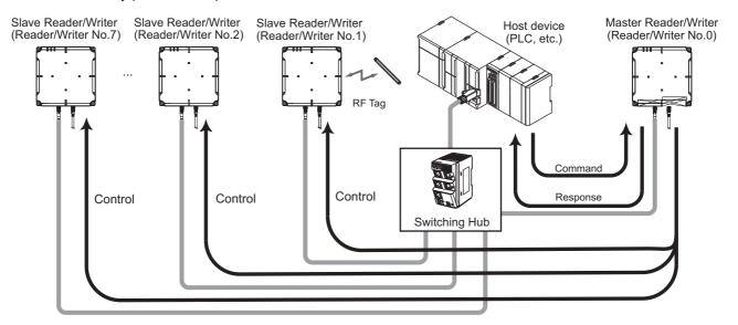
In the Multi-Reader/Writer function, the slave Reader/Writers connected to the master Reader/Writer are differentiated by the following Reader/Writer numbers.
