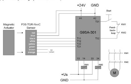
Wiring example with reed switch and G9SA controller: (wiring colors are shown for flyinglead – types)
