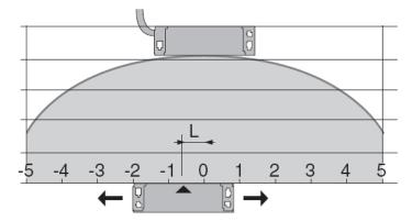
5 mm misalignment tolerance after setting
