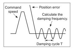
• The damping frequency in the figure is calculated with the following formula:
