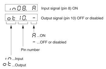
• Displays the status of the control input and output signals connected to CN1.
