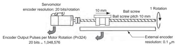
External Encoder Output Pulse Per Motor Rotation (Pn325)  $10 \text{ [mm]} / 0.1 \text{ [} \mu\text{m/pulse]} = 100,000 \text{ [pulses]}$
