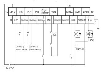
\*1. CW and CCW limit input signals can also be input through Input Units. The signal for the CW/CCW limit inputs in the CJ1M are as follows: CW: A540.08, CCW: A540.09 for pulse output 0 and CW: A541.08, CCW: A541.09 for pulse output 1. Accordingly, the actual inputs can be used as the CW/CCW limit by outputting the flags below in the ladder program.
