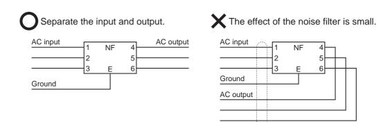
• Use twisted-pair cables for the power supply cables, or bind the cables.
