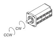
• Regarding the motor rotation direction, when seen from load-side axis, clockwise is referred to as CW and counterclockwise as CCW.
