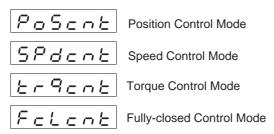
• Displays which control mode is being used: position control, speed control, torque control, or fullyclosed control.
