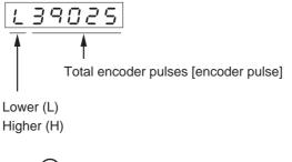
Press ( to switch between Lower (L) and Higher (H).
