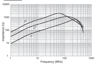
Refer to the following sections for the dimensions and impedance characteristics of the ZCAT3035-1330: "External Dimensions" (P.4-46) and "Impedance Characteristics" (P.4-47).
