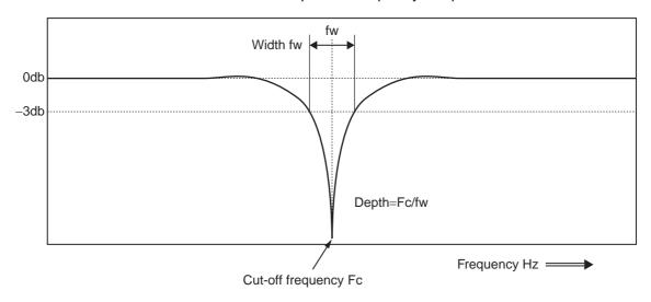
If machine resonance occurs, use this notch filter to eliminate resonance.
