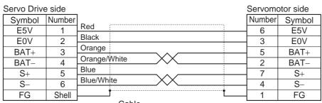
[Servo Drive side connector] Connector model
