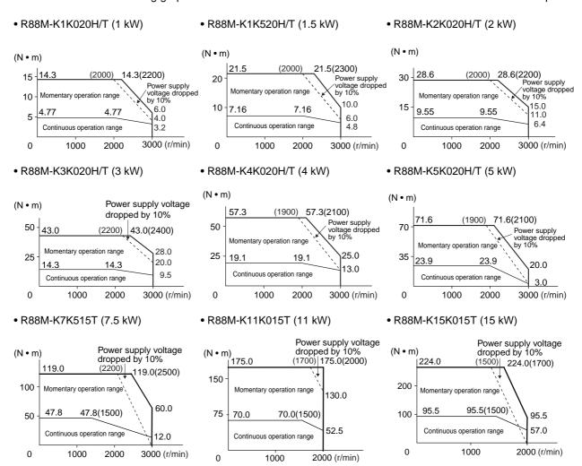
Note 1: The continuous operation range is the range in which continuous operation is possible. Continuous operation at the maximum speed is also possible. However, doing so will reduce the output torque.
