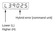
Press to switch between Lower (L) and Higher (H).
