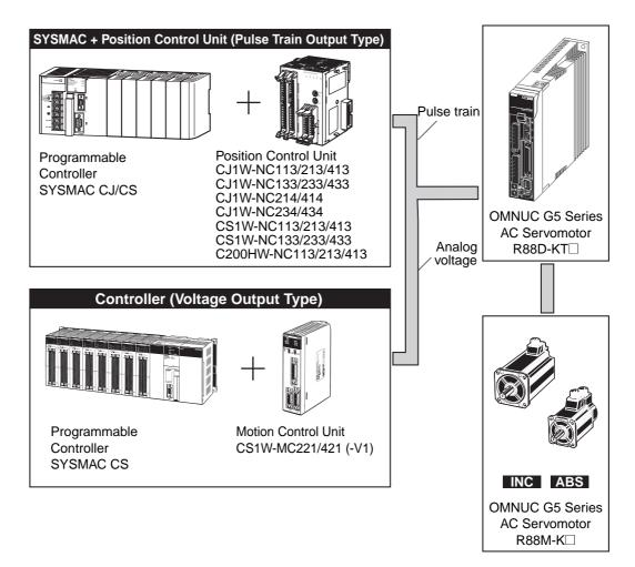
The following units support a motor with absolute encoder: CJ1W-NC214/414 CJ1W-NC234/434 CS1W-MC221/421 (-V1)
