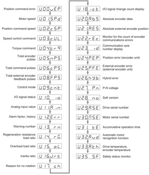
When sis pressed, the display position will move in the direction of the arrow.
