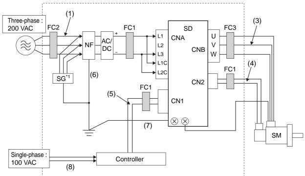
Note. The main circuit power supply input terminals are L1 and L3. Connect the positive line to L1 and the negative line to L3.
