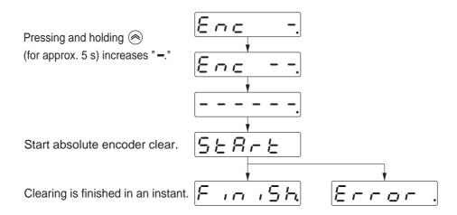
Note. *Error* will be displayed if absolute encoder clear is performed on an incremental encoder.
