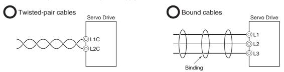
• Separate power supply lines and signal lines when wiring.
