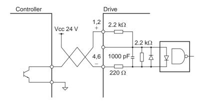
• External control power supply (200 kpps maximum) (+CW: 3, -CW: 4, +CCW: 5, -CCW: 6)
