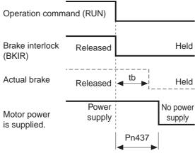
•Make the setting as follows to prevent the machine (workpiece) from moving or falling due to the delay time in the brake operation (tb).
