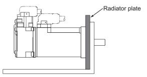
• The temperature rise depends on the mounting part materials and the installation environment. Check the actual temperature rise by using a real Servomotor.
