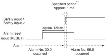
\*1. Alarm No. 99.0 will occur if at least one of the input photocouplers for safety inputs 1 and 2 is turned from OFF to ON.
