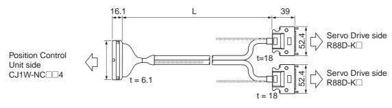
Cable for line-driver output for 1 axis
