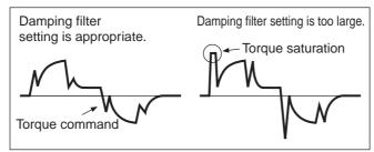
When the Damping Frequency 1 (Pn214) is set, reduce the setting if torque saturation occurs or increase the setting to increase operation speed. Normally 0 is set.
