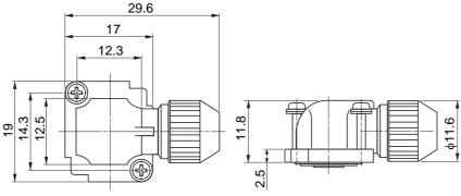
Angle plug model JN4FT02SJ1-R (Japan Aviation Electronics)
