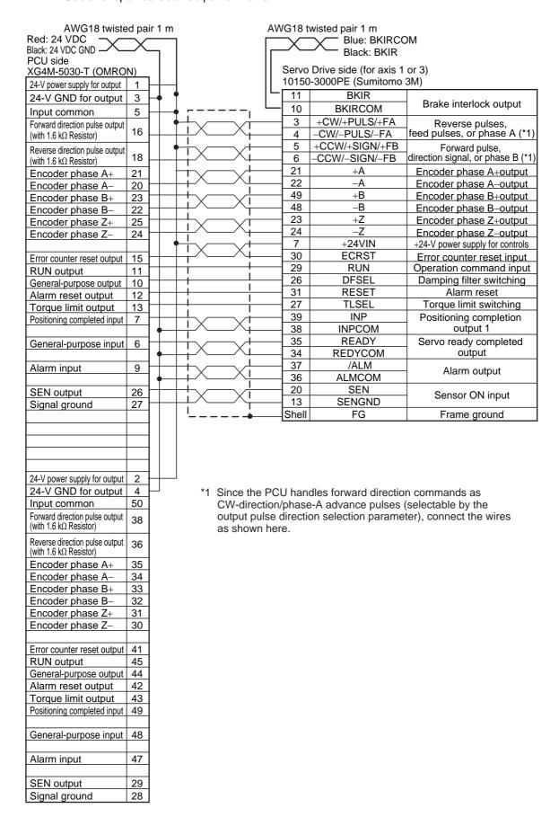
Cable for line-driver output for 2 axes
