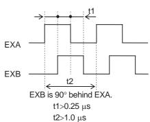
\*2. These are the feedback speeds from the external encoder at which Servo Drive can respond. Check the external encoder operation manual for its maximum output frequency. For example, the maximum speed when an external encoder with a resolution of 0.01  $\mu$ m is used for the serial communication type is 0.01  $\mu$ m  $\times$  (400  $\times$  10<sup>6</sup>) pps = 4.00 m/s. An overspeed error protection is generated, however, if the motor shaft rotation speed exceeds the maximum speed.
