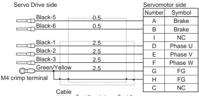
$2.5 \text{ mm}^2 \times 4\text{C} + 0.5 \text{ mm}^2 \times 2\text{C}$
