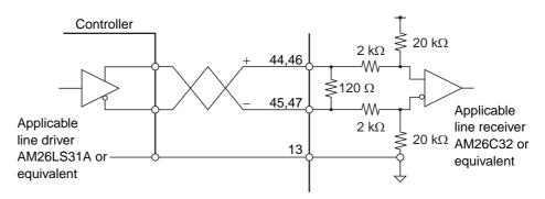
• The shielded twisted-pair cable should not exceed 10 m in length.
