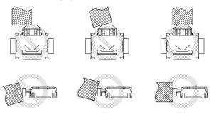
Do not operate the plunger from the side. Doing so may deform or damage the Switch.
