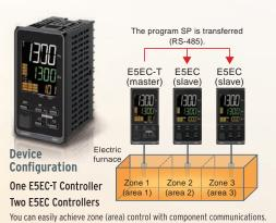
You can easily achieve zone (area) control with component communications. RUN/RESET status of master TC and slave TC link to achieve consistent furnace temperatures in order to improve productivity and reduce lead time.
