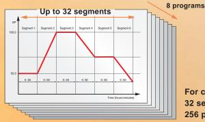
For complex temperature control, you can set up to 32 segments in each program, for a total of 256 program segments.
