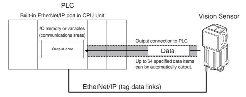
To output data, you must specify in advance the data to output (up to 64 items) after the measurements are executed.
