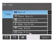
When registering multiple inspection items, press the inspection item number after 1.--- and set it in the same way.
