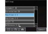
If the inspection item allows multi-point output, press the number ([0] to [30]) of the inspection result for which to output the data from the list of inspection results.
