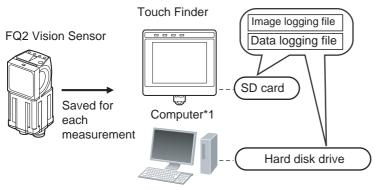
\*1: Image data and measurement data can be logged in the same way as for the Touch Finder by installing the PC Tool for FQ.
