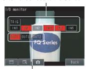
Output Signals (OUT0, OUT1, and OUT2) Signals that are displayed in red are currently being output from the Sensor to the external devices.
