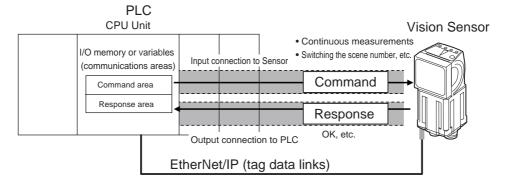
To send a control command, you write a control command to the command area (i.e., a variable or I/O memory address in the PLC) that is specified for the output tag, and then turn ON the Command Execution (EXE) Bit. As a result, the control command is sent through the input connection from the PLC to the Vision Sensor.
