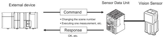
The external device sends a command as an ASCII string (e.g., "MEASURE" for a single measurement). The Vision Sensor then returns a response such as "OK", "NG", or some value.
