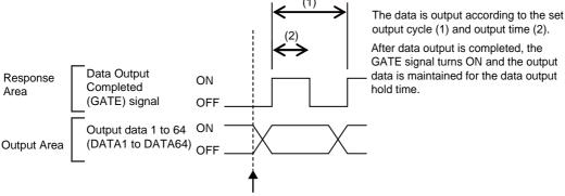
Here, the Vision Sensor ends measurements and can output data.
