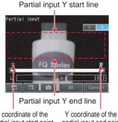
Y coordinate of the partial input start point partial input end point
