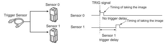
Sensor 0 immediately begins image input when the trigger is input. Sensor 1 begins image input after the specified time has passed.
