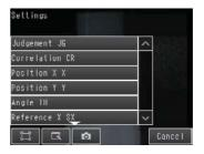
If the inspection item allows multi-point output, press the number ([0] to [31]) of the inspection result for which to output the data from the list of inspection results.
