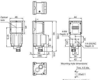
Tightening torque: 1.2 N·m
