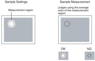
If a Sensor with a Monochrome Camera is connected, the average density in the measurement region is measured and the density deviation is used for judgements.
