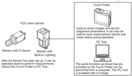
FQ2-series Vision Sensors are available in two different models. There are also Sensors with C-mounts that allow you to change the lens, and Sensors with Built-in Lighting. The differences are given in the following table.
