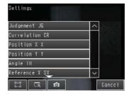
5 If the inspection item allows multi-point output, press the number ([0] to [30]) of the inspection result for which to output the data from the list of inspection results.
