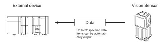
You must specify in advance the data to output (up to 32 items) after measurements. That data is sent to the external device in either ASCII or binary format through a continuous serial connection. There is no handshaking from the external device to confirm if it can receive the data.
