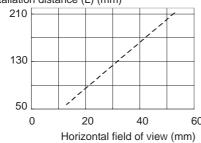
The optical chart indicates the horizontal field of view. The vertical field of view depends on the model as follows:
