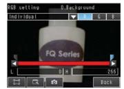
4 Set the upper and lower limit values of the brightness range. (for Sensors with Monochrome Cameras (or after a Color Gray Filter))
