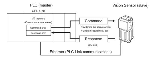
After you write a control command to the specified Command Area in the I/O memory of the PLC, you can turn ON the Command Execution (EXE) Bit to send the control command to the Vision Sensor via Ethernet. The Vision Sensor executes the control command and sends a response back to the PLC via Ethernet. The PLC stores the response in the specified Response Area in I/O memory.
