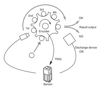
If you set the [Number of delay] parameter to 4, the measurement result output is delayed by four TRIG signals.
