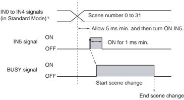
\*1: In Expanded Mode, specify scene numbers 0 to 15 using the IN0 to IN3 signals.
